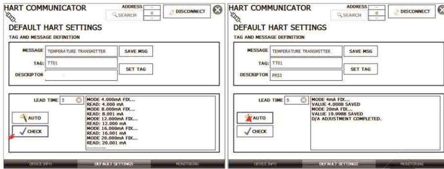
Fig. 26 - Checking / Adjusting the mA HART® Transmitter Output
