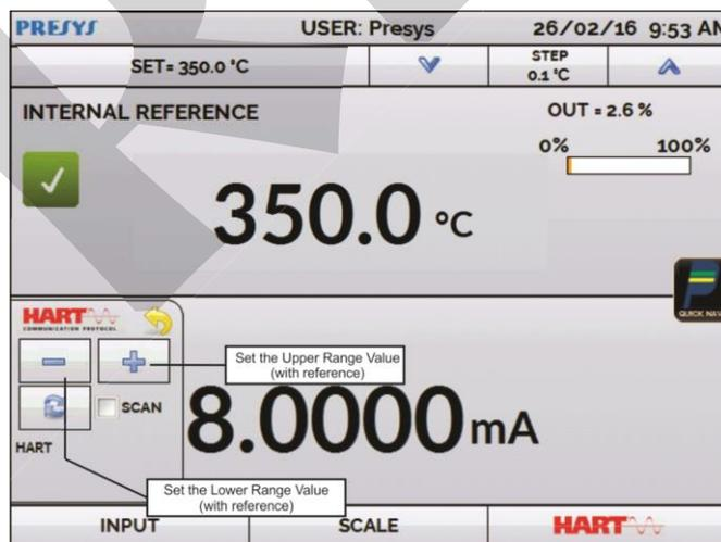
Fig 24 - Quick Hart® Adjustment with Reference
