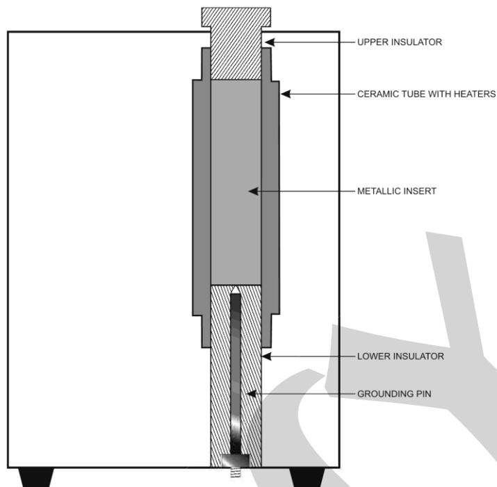
**Fig 2 - Schematic View for Insert Mounting**
