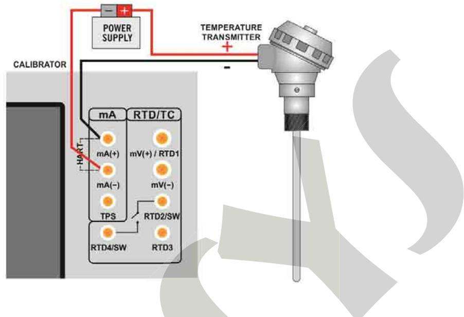
**Fig. 22 - Transmitter Powered by an External Power Supply
