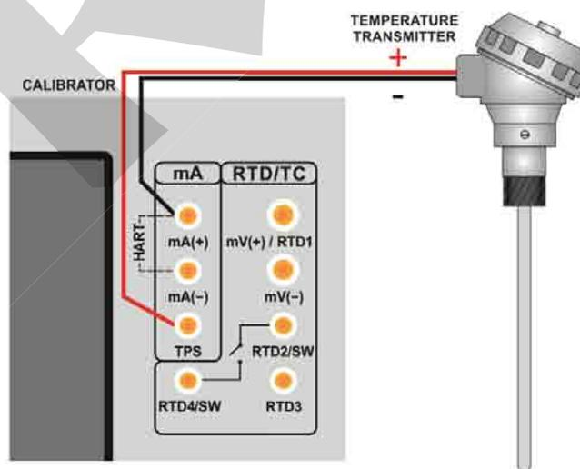
**Fig. 21 - Transmitter Powered by the Calibrator Itself (TPS)
