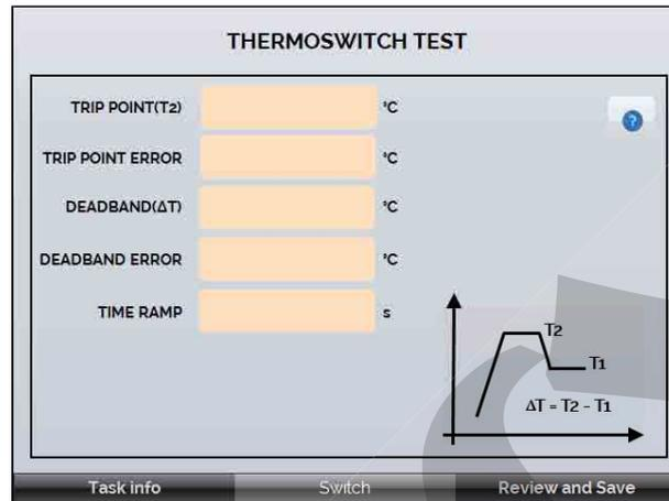
**Fig 29 – SWITCH Task Parameters**
