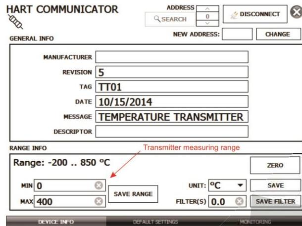
Fig. 23 - Adjusting the measuring range of the HART® transmitter
